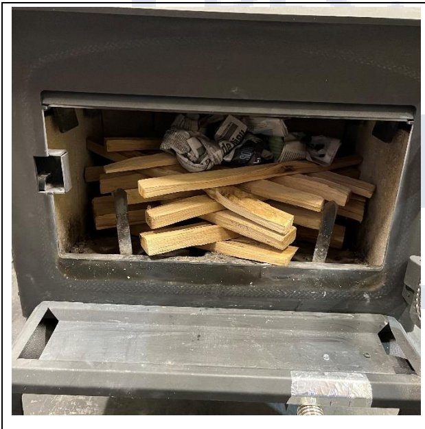
Kindling & Start-up Loaded in Stove
