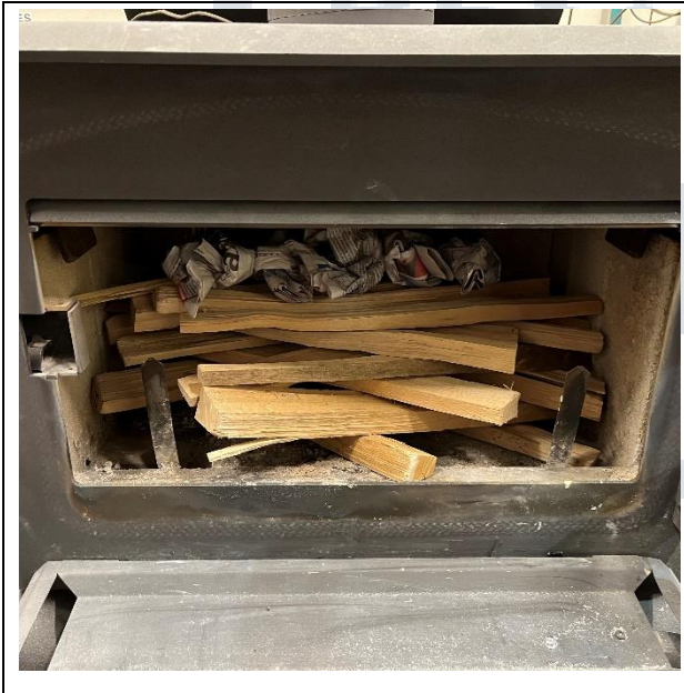
Kindling & Start-up Loaded in Stove
