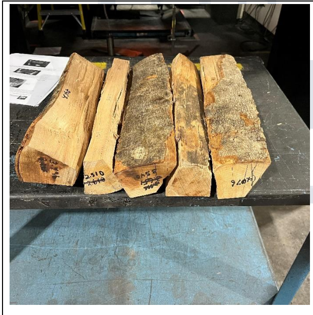
Medium Fire Fuel Load
