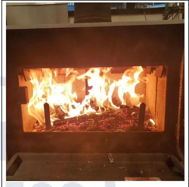
Residual Start-up Fuel Coal Bed – Post Rake
