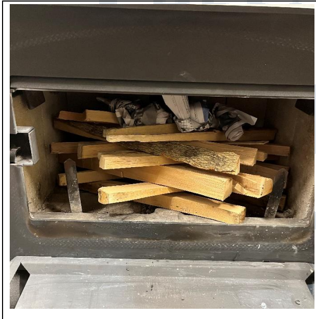
Kindling & Start-up Loaded in Stove
