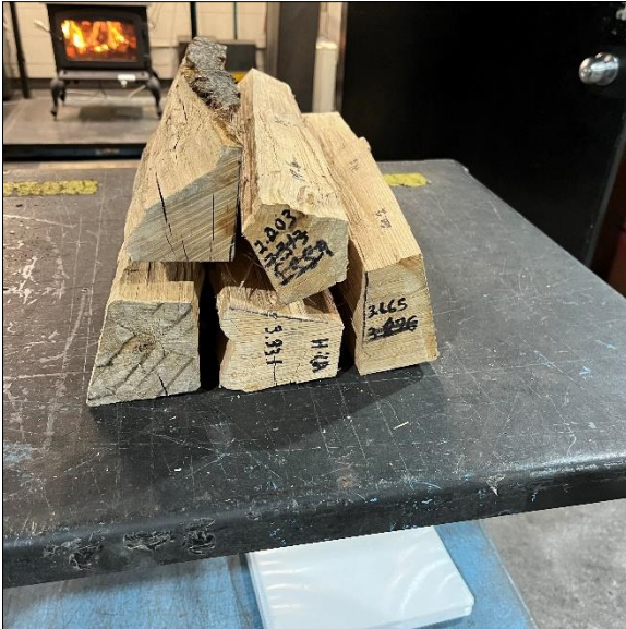
Typical High Fire Load
