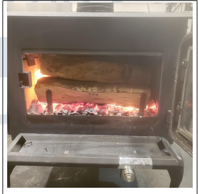
Medium Fire Fuel Loaded
